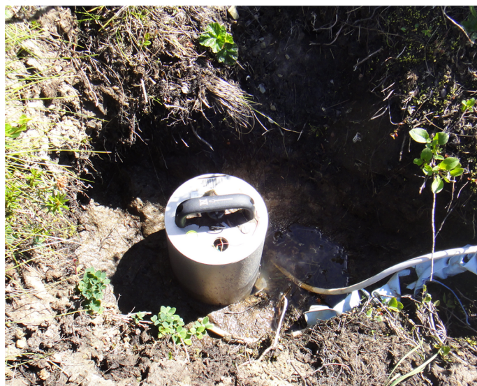
▲ Figure 5. Remains of MMEP station MM31, at Cache Lake in Northwest Territories, Canada. The station was installed on 2016-08-15 and stopped collecting data on 2016-08-27. This bear encounter appears as MM31/16 in the R4 and B6 box in © Table S2. (a) View of site on 2017-07-17. (b) View of partially unburied sensor. Because of time constraints and marshy substrate, the 3T seismometer was placed before the pier was fully cured, resulting in the sensor feet becoming mired in concrete. The cable port on the 3T consequentially broke off during the bear attack, exposing the internal electronics and destroying the sensor. The color version of this figure is available only in the electronic edition.
