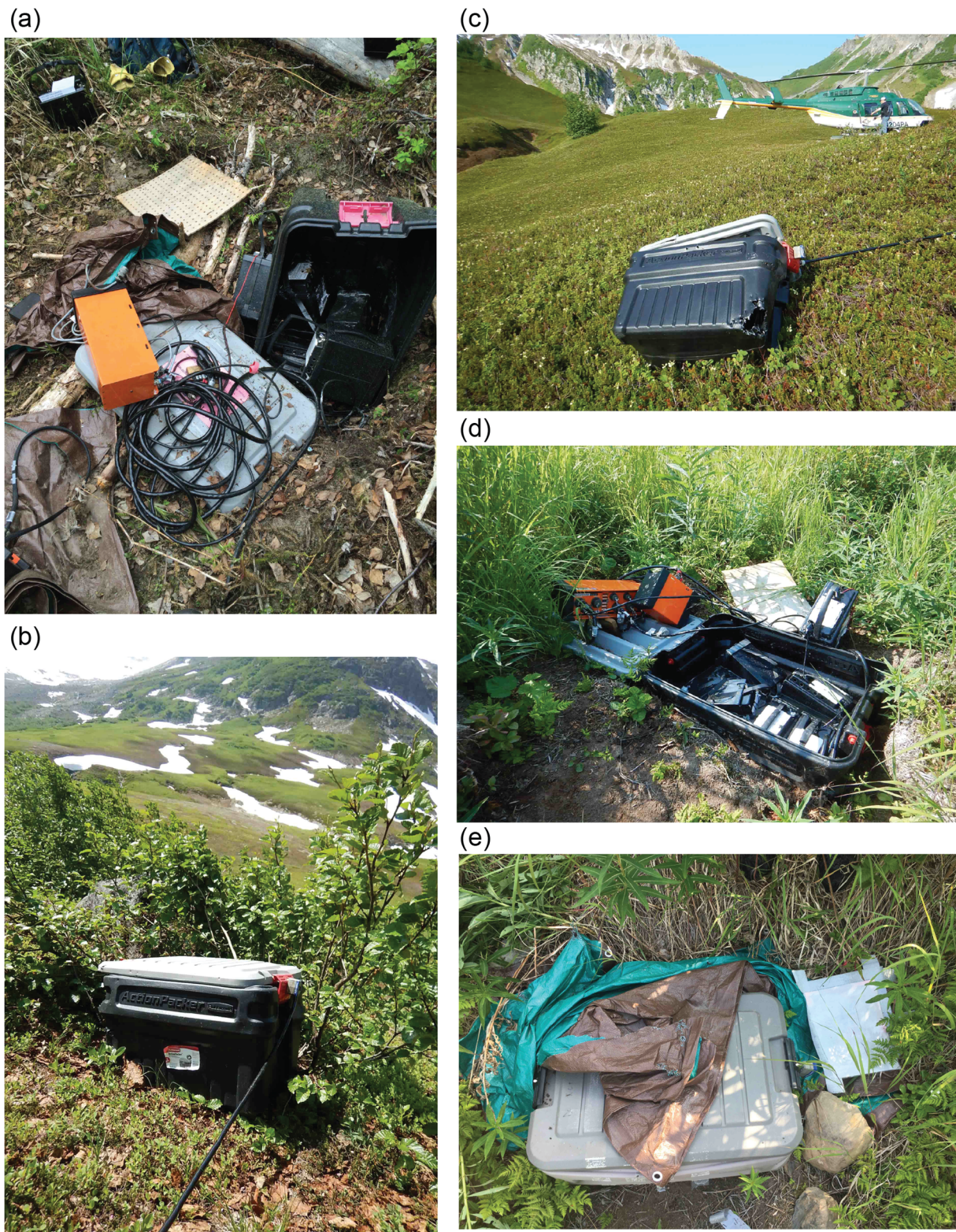
▲ Figure 4. SALMON station outages caused by bears. These photographs are associated with the following labels in Table 3: LTUW/15 (B6), HLC2/15 (B6), HLC1/16 (B6), HLC3/16 (B5), HOPE/16 (B5). (a) LTUW on 2016-05-18. The outage occurred on 2015-07-15, 12 days after installing the station. (b) HLC2 on 2016-07-19 (outage 2015-10-03). The sensor cable had a single, deep bite mark and the Q330 recording system was short circuited. (c) HLC1 on 2017-07-12 (outage 2016-09-30). The box is tethered by the sensor cable; one battery had been removed from the box. (d) HLC3 on 2017-07-12 (outage 2017-05-19). (e) HOPE on 2017-07-16. Removal of tarp and deformation of the box allowed water to fill the box, causing a power outage on 2017-06-12, >12 months after servicing. The box top had tooth holes. The color version of this figure is available only in the electronic edition.
